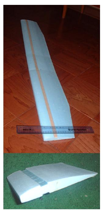
Cutting guides must be made and carefully positioned on the ends of the foam slab.
