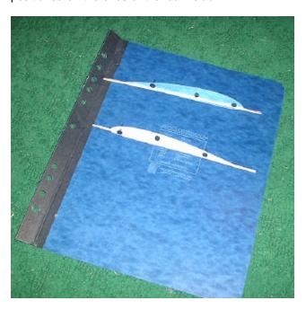
Grooves for spars, etc. are best made after the initial cut. Dick has used a homemade fixture with a short loop of music wire bent to the shape of the desired groove, powered by the same battery charger, to cut spar grooves.
