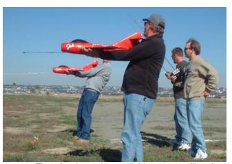
The fuselage is available as a fiberglass molding; the wing and tails are balsa over foam. The fan units are commercially available. There was a recent article on these models in S&E Modeler. I gotta have one of these airplanes!
