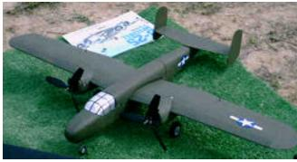
His second airplane was a B-25 at about 30 inches span. This airplane has a fixed gear but had no problem with the rough surface. In fact the flight performance was sparkling. The airplane was powered by two Light Stick motor / gearbox assemblies (less than \$20 each) it had a built up balsa / tissue wing. The fuselage and nacelles. were carved from foam, covered with tissue and painted.
