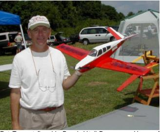
Pat Taggart flew his Beech V-tail Bonanza, a House of Balsa kit. The plane has a speed 400 motor with a Graupner 2.33:1 gearbox, Graupner Cam 9x5 prop, and Astro 215D controller.
