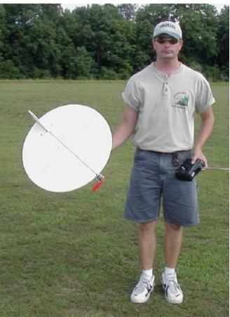
Rich Bourassa shows his plane with a wing made from a round piece of Styrofoam. The plane is powered by a Titanic Airlines 280 motor with a 3:1 gearbox, and uses a 7x6 prop and 7 batteries 500.
