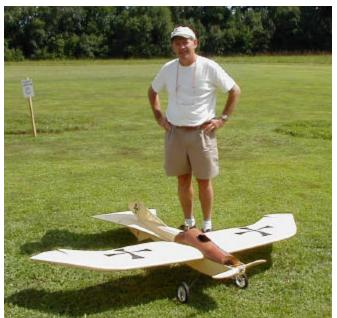
Pat Taggart placed #1 in the Scale contest with his Balsa USA Taube 90 size kit. The Taube has an Astro 40 with a 3:1 super box, 16x10 Master Airscrew prop, and 22 batteries 2000.
