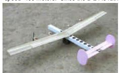
thought I would build a "test horse" to try it out. Shown here is the test horse which uses a foam glider wing of 76 inch span and a drainpipe fuselage. The actual B-24 fuselage is shown in the background. One design feature of the Bristol is a soft EPP foam nose. It has saved the model many times as I have learned to fly. I can't decide whether to use it on the B-24. I suppose eventually you design them to fly not crash. Don't think I am there yet. **Dave**
