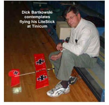
I flew my Litestick a number of times. Most flights resulted in contact with the walls or furniture and a failure of some kind. However, the Litestick is easy to fix and a shot of CA and accelerator usually does the trick.. This model has a replacement motor with a higher gear ratio and a bigger 12 x 8 prop. It seems particularly well suited to slow indoor flying.
