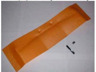
There was a molded foam-sheet 17-inch wing with a flat center section and dihedral tip sections, a minute N20 motor and 3 inch prop. "Should be able to build a model light enough to fly with two 50 mah NiCad cells". "There are a variety of Nocal profile scale designs on the web, why not make a Hurricane?"
