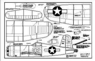
Scale it up to 16 inches span, easy. Print it out and cut and glue the wing. Hey, I have started to build it! Quick cut out the stab and fuselage from thin sheet foam. Need to put some doublers in the usual forward fuselage area, how about that, I can bury the motor, add some wire and velcro. Wow, its finished. Wonder if it will fly.
