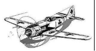
The swirling prop wash effects can induce rolling and yawing from interference with the airframe
