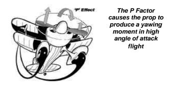
However, since the Cub is climbing with its nose high relative to the airflow, the descending blade on the right sees a bigger angle of attack AND a slightly higher airspeed than the rising blade on the left, and so the blade on the right makes more thrust than the blade on the left. This tends to yaw the airplane to the left.
