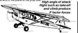
Meanwhile the blade on the left side is rising. Its angle of attack is a function of the pitch angle MINUS the angle between the inflow and the propshaft. Its local airspeeds along the blade are a function of the rotational speed at each location MINUS the component of the inflow airspeed that acts in the plane of the disk.
