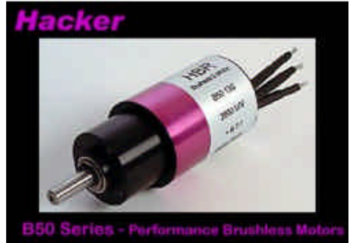
This Hacker brushless motor and 6.7:1 planetary gearbox weighs just 9oz and handles 700 watts, or 1 horsepower. The rotor turns up to 80,000 rpm.
