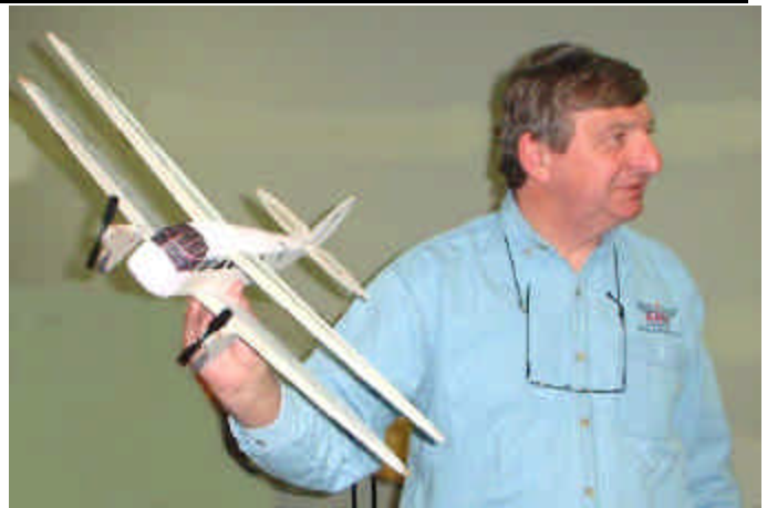
Dave also showed his Hobby Club Puma- E-Fluffy ARF electric glider. Weight is 18 oz., speed 400 6V with 4.5:1 planetary gearbox, 7 cells and 14" x 9 folding prop.
