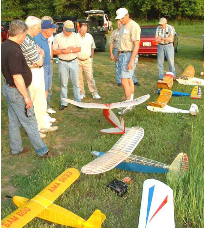
Dick Bartkowski explains his electric powered Pacer 'C' Old Timer Limited Motor Run competition model. An inexpensive Speed 600 motor and belt drive speed reducer powers it.
