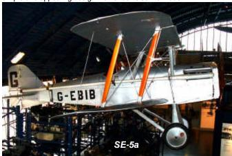
The Science Museum's SE-5a is one of a number that were salvaged after WWI and converted to the new technique of skywriting. Note the asbestos lagged exhaust pipe that was probably to enhance the smoke generation. Certainly a different color scheme. There is an SE-5a in military colors in the RAF museum.
