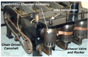
Notice, the Wrights used chain-driven high mounted camshaft acting directly on the rocker arms. Spark ignition was continuous, not timed, allowing the plugs to be gang-fed by a copper strip.
