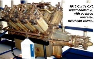
As engines improved it became obvious that aerodynamic and thermodynamic efficiency was important to lightweight fuel-efficient engines. Make them efficient and they will be smaller and lighter for the same output.
