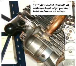
This close-up of one bank of cylinders on an air-cooled 1916
