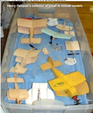
His earlier very small models were powered by a whole range of tiny CO2 motors, initially built by the legendary Bill Brown of Brown Jr. fame. Indeed, Henry still uses CO2 motors, now built by Gasparin in the Czech Republic. The latest motor will have a cylinder bore of one millimeter, 0.040 inches, just over 1/32 inch!
