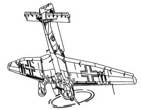
If we ignore the stub sections next to the fuselage, the Ju-87 Stuka has about 9 degrees of dihedral per side, measured at the chord line of the airfoil. The stub sections
