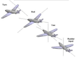
In general, just a few degrees of dihedral are sufficient for adequate roll stability, but to use rudder plus dihedral for roll control generally requires much more dihedral. In my experience, a general rule of thumb for adequate roll control in a typical sport model is at least about 8 degrees of equivalent dihedral per side.
