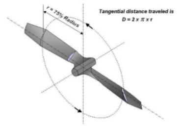
If we multiply that by the revolutions per second that the prop is spinning, we get the velocity in the plane of the prop disk of that location on the blade. We call this the "tangential velocity".
