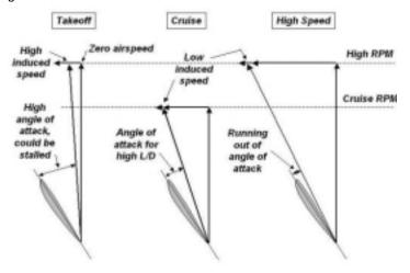
At higher airspeeds, there is more air flowing through the prop, so that air needs less acceleration to convert the power into thrust. This means lower lift coefficients, and therefore lower angles of attack. At the highest speeds the increased airspeed causes the prop angle of attack, and thrust to reduce until thrust equals drag at maximum speed.
