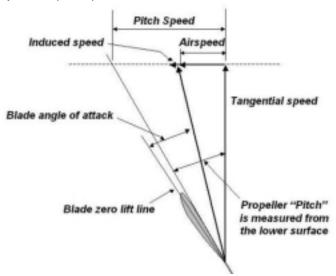
Now let's put some numbers into all this. In the table over leaf are the blade pitch angles for various propellers. We use the definition pitch-to-diameter ratio: P/D, for the propeller because it is this ratio that determines the blade angles.
