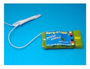
It weighs only seven grams, about ¼ ounce but has all the high tech signal processing and features an indicator lamp, which indicates the number of glitches filtered out during the last flight.
