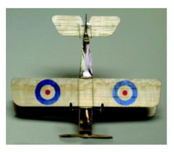
The 4 X 8-mm. (0.16 X 0.31-in.) electric propeller motor comes from a pager vibrator and is geared down 1:3.5 to drive the 1.6-in.-dia. numerically machined maple prop. Current consumption is about 110 milliamps from the 3.2-volt 20-milliamps-hr. lithium polymer battery weighing 0.7 gm. "The battery wasn't doable five years ago."
