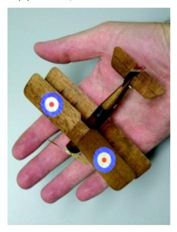
Key technologies making it possible are a novel homemade actuator powered by shape memory alloy wire, and a tiny high-performance battery. The aircraft has flown 4 min. at a time and should be able to go 10-15 min. on a charge.
