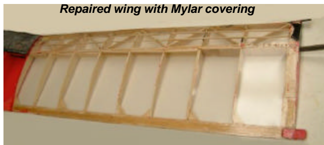
Repaired wing with Mylar covering
