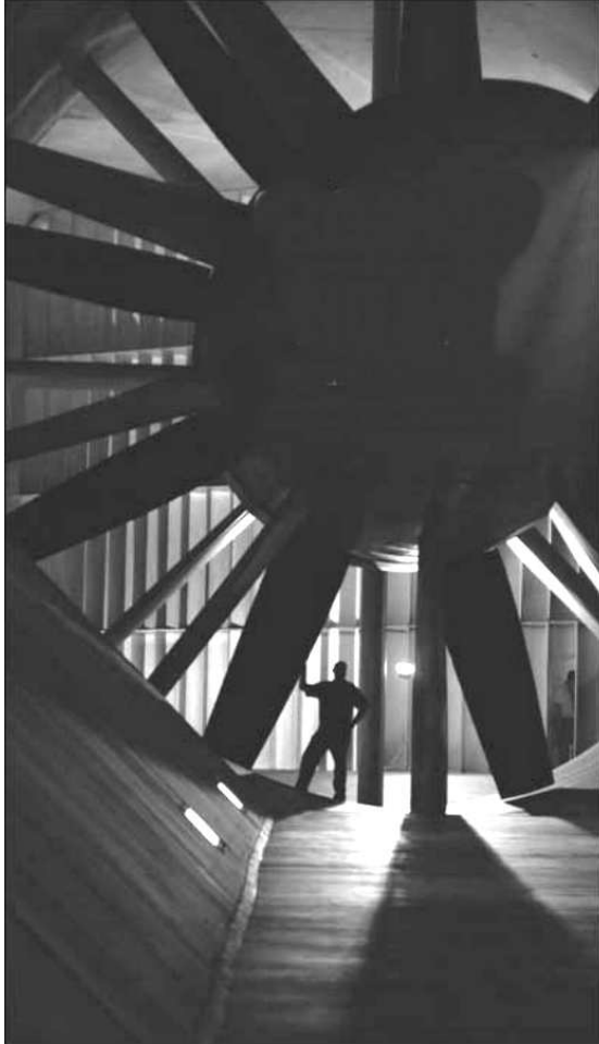
The Boeing Philadelphia subsonic wind tunnel is the largest privately owned wind tunnel in the United States. The nine-blade fan (shown here), measuring 40 feet (12 meters) in diameter, can generate up to 15,000 horsepower and speeds greater than 220 knots. Since opening in 1968, the facility has logged nearly 70,000 test hours.
