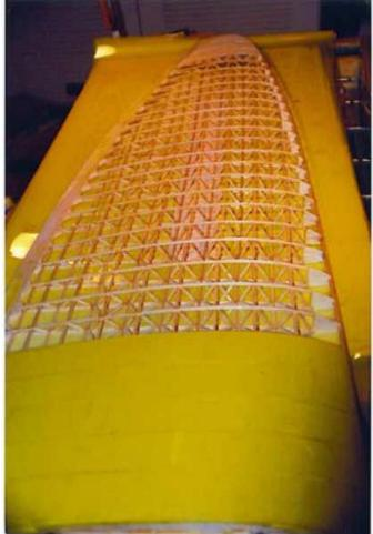
Don says; the Valkyrie should really be recovered after repairing the wing spars. Note that those spars are small, 1/8sq. spruce, but there are so many glue joints that the whole wing should be checked for solid joints as I did years ago when I recovered the wing -- as should the tail. The best covering would be SAM Span [polyspan] because the dope increases
