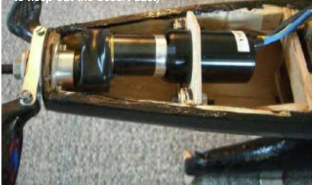
Dave's big Stardust Special Electric Texaco propulsion system; a Neu motor with Maxton planetary gearbox mated to a 2.33:1 spur gear reduction (wrapped in tape to keep out the desert dust)
