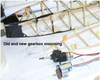
The old Wakefield had an MP Jet 5:1 gearbox that mounted on three lugs arranged in-plane so that they could fasten to a semi-bulkhead at the second bay. I broke this joint many times over the four years it was used in the original model, but each time I fixed it easily and when fixed it held the desired alignment. Here is an earlier fix where the whole forward fuselage was replaced.
