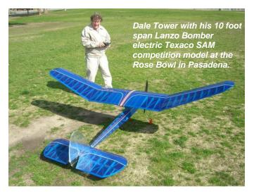
This model is much bigger than the normal full-sized Bomber. It has about 1700 sq inches wing area and a span of nearly ten feet. Dale has set it up with twenty of the Sanyo N 1000 SCR NiCad cells from a batch of 100 I bought on eBay. He had to chase down a special ESC to operate at this voltage. Apparently the Chinese are making these and many other ESCs at this time and Dale has found a source through which he can get them at really low prices.
