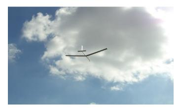
It floated out of my hands into the modest breeze but control was initially a handful as the fuselage was very soft in torsion. When Dale put rudder control input the fuselage would twist and take out much of the control force. It took a little while for him to sort it out following which it floated around with practically no power input. Watch this space to follow his progress.
