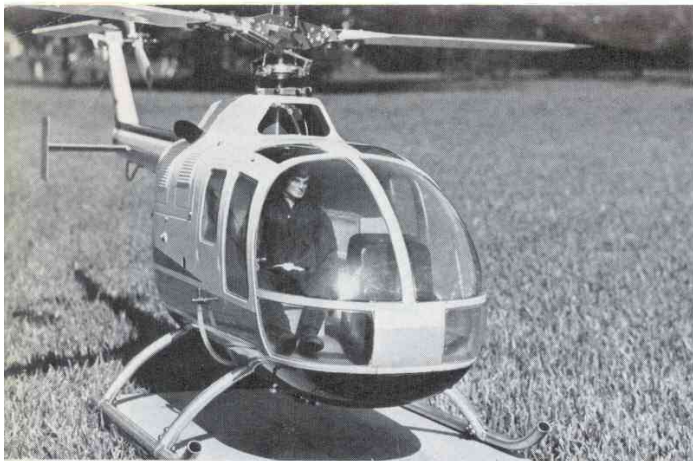
Author Rock's Froude-scaled Boelkow BO-105 and its main rotor. This 11-lb model has a 54-in-diam rotor and is powered by a Webra 61 engine. As seen in photo at right, the main rotor features a Hiller bar, collective pitch control and Chinese-top weights to minimize collective control force.
