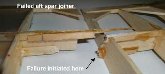
You can see the spar and joiner failed completely at the root and the outboard end, and there is evidence of a poor glue joint to the shear web. The upper spar joiner shows a failure mode that you would expect from the upward failure motion of the wing after failure of the lower element. The forward spar exhibits failure modes consistent with wing failure initiating elsewhere; the aft spar.
