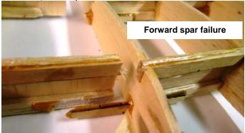
The lower spar failed by shearing cross grain between the joiner and the spar. This shows joiner and spar were basically sound and the glue joint good. The upper spar, like with the aft spar assembly, failed in bending as the wing failed upwards.
