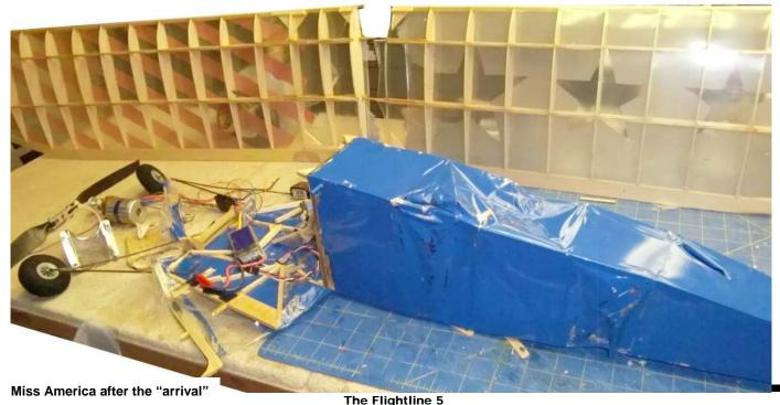
bays. The tail was largely intact as were the pushrods although one of the servos had broken loose from its mounting. The nice "between the wars" cowling was completely destroyed back to the motor bulkhead, although the sheet aluminum flashing motor mount was largely intact.
