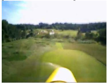
The first thing you notice is the "shuttering" or interference of the prop passing the camera and the camera frame rate. I suppose you could figure out the rpm from the direction of the pattern movement and the spacing of the prop lines.
