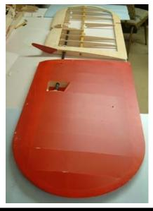
The LH horizontal had departed the aircraft with a failure of the pivot/spar graphite tube flush with the root rib. The other side, the damaged part, remained attached to the aircraft through the pivot/spar remaining half inserted into its socket in the fuselage and the pitch horn attachment to the servo. It had damage in a line diagonally across from front to back; severing the leading edge, trailing edge and the spar.
