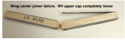
The failure is interesting for two findings, first the RH upper spar cap became un-bonded from the plywood shear member.
