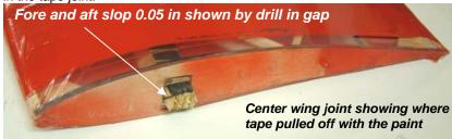
The remaining very interesting finding is that the center wing joiner failed. You may remember that I structurally tested the entire wing spar/joiner assembly before building the wings. So how could this have happened?
