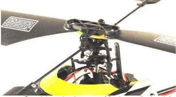
One of the main advantages of fixed vs. collective pitch system is that the mechanics of the head are considerably simpler, reducing the cost of the helicopter, and making the system more tolerant of the abuse that a beginner machine typically encounters.
