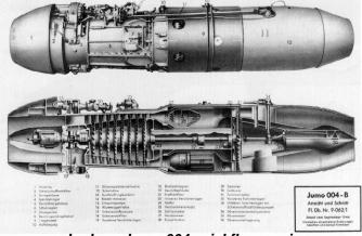
Junkers Jumo 004 axial flow engine
