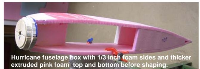
Hurricane fuselage box with 1/3 inch foam sides and thicker extruded pink foam top and bottom before shaping.
