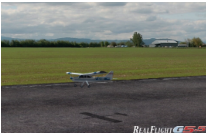
If you're not down by now, go to 100% throttle while you still have time to make another go-around. Otherwise you risk running out of runway. Runway behind you is useless!
