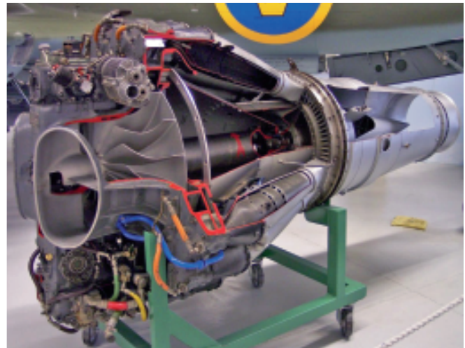
Note the diameter over the combustion chambers in relation to the jet exhaust outlet diameter. Whittle's engines incorporated centrifugal compressors like this one;
