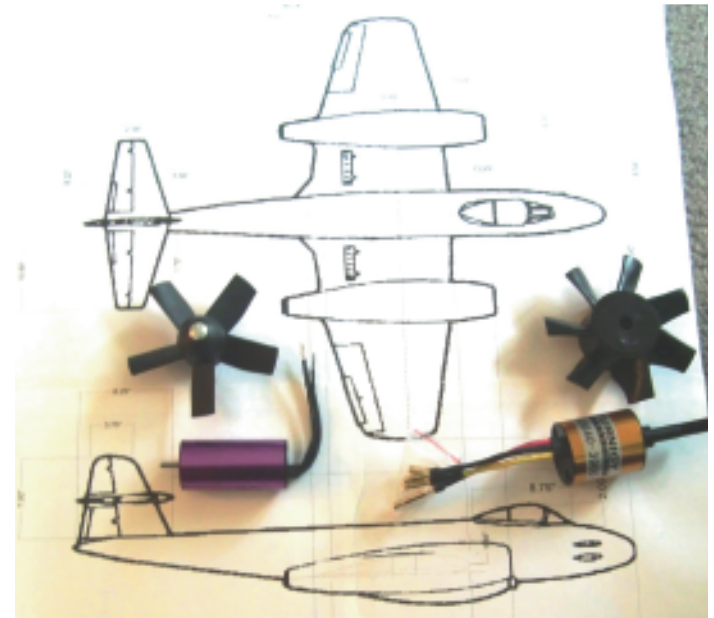
The "cheapie" fan on the left came with an Aerowind 1900 Kv, 28 mm diameter motor good for 26 amps I bought a Turnigy 3640 3900 Kv motor from HobbyKing for the Germa fan. Since I had no experience running Motocalc with EDFs thought I should bench test them first so I made a simple mount to attach to a 2 x 6 clamped in a big vice.
