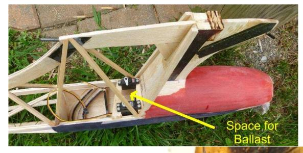
Now the challenge was to make a piece of ballast that fit this space and weighed 15 oz. This could only be satisfied with a molded led piece. So I set about making a mold from some pieces of wood into which I would melt old lead tire weights. Fortunately my son works for Subaru and we regularly harvest the crop of castoffs.
