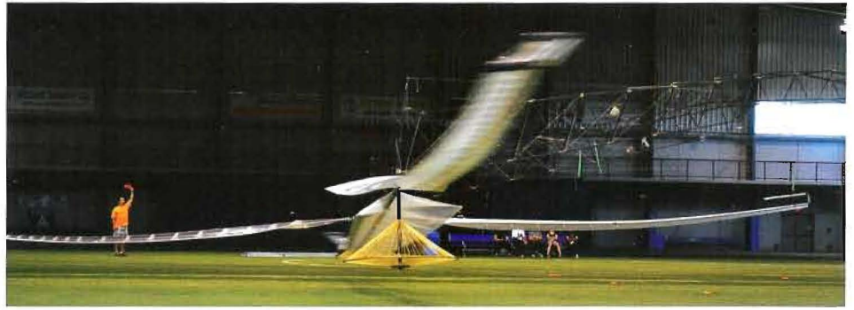
During one of several late August tests, Atlas takes flight. Aeroelasticity, trimming the four rotor systems and gyroscopic precession were all interesting challenges. AHS photo.
