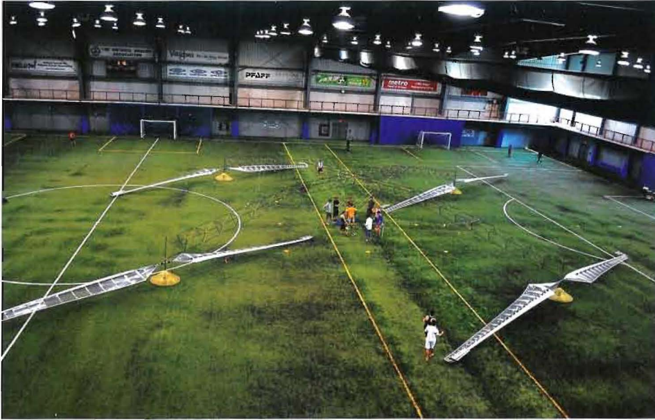
AeroVelo's Atlas is the largest human powered helicopter to have ever flown and the first one in Canada. AHS photo.
