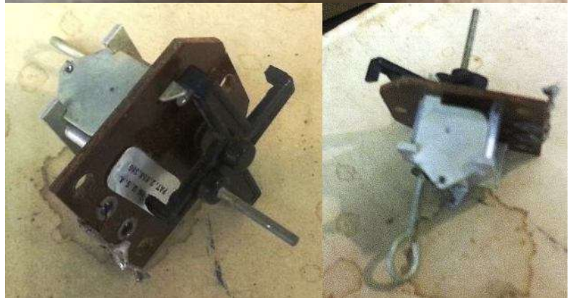
Above; Al's pulse single channel radio with a rubber band powered escapement for control.
