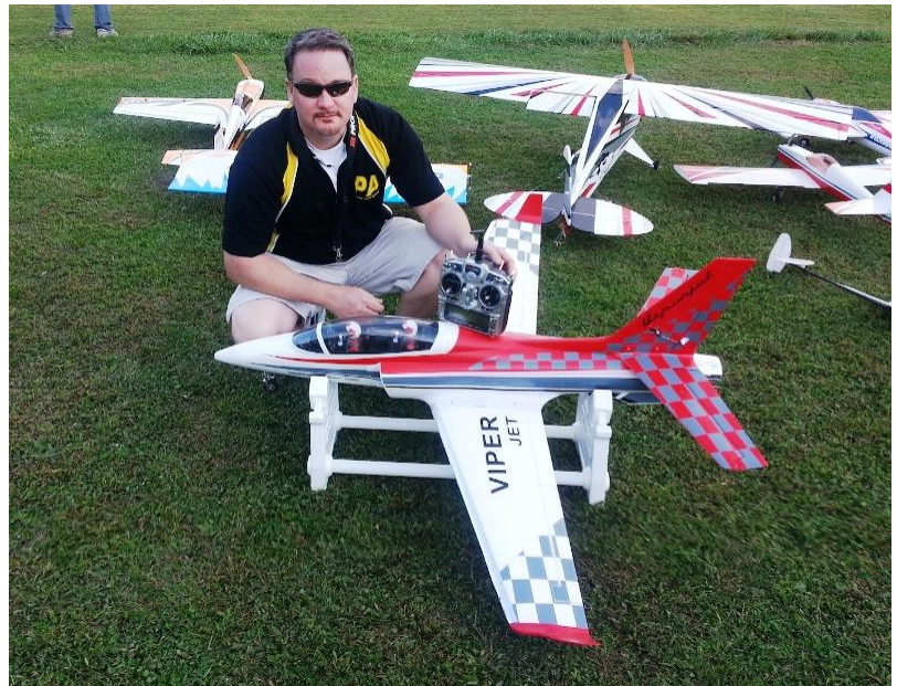
Jeff with new jet; A Taft Hobbies 90mm EDF Viper. It runs on 6S 5300mah packs.
