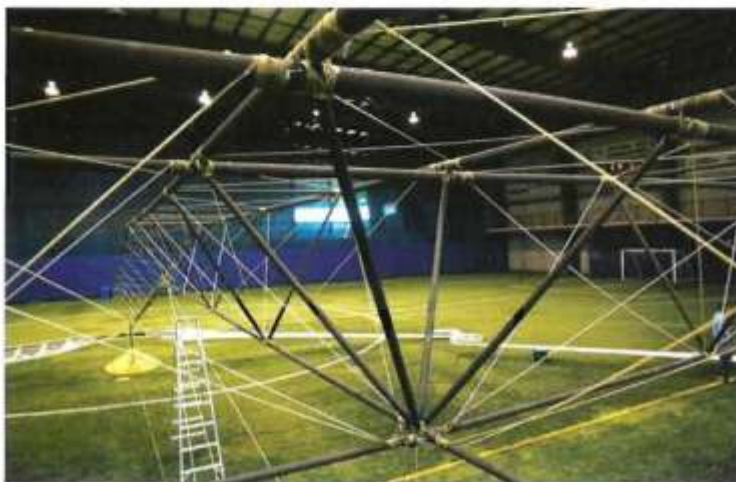
Close-up view of the center of the Atlas trusses. (AeroVelo photo by Jake Read)
