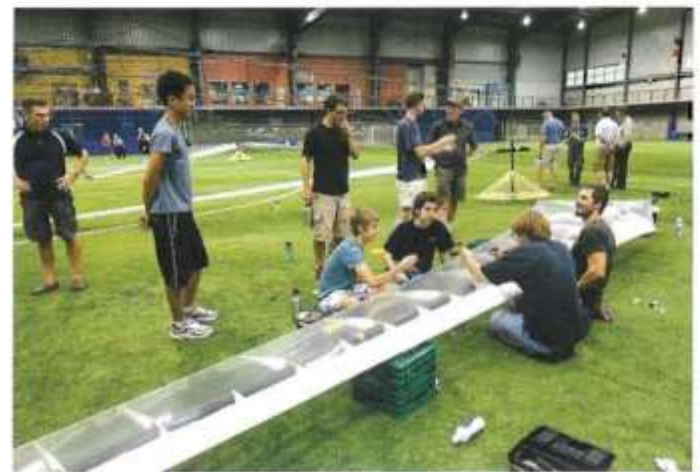
Repair of the rotor mid-spar after a September 1, 2012 impact. (AeroVelo photo by ckmmphotographic/Mike Campbell)
