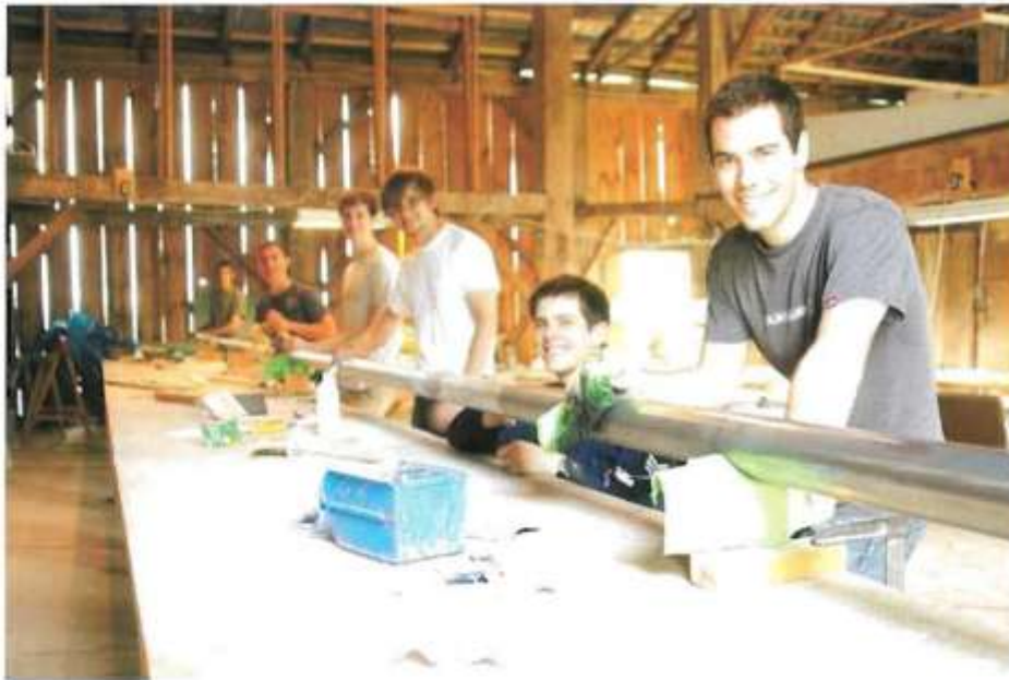
Robertson and team fairing the rotor spar mandrel in their barn workshop in May 2012. (AeroVelo photo by Jake Read)
