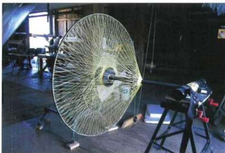
Atlas rotor spool on a test stand in the old barn in July 2012. (AeroVelo photo by Todd Reichert)
