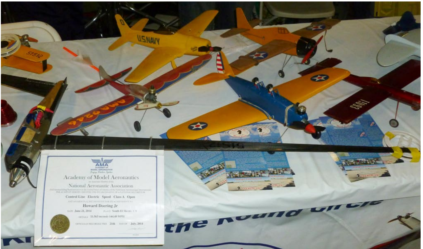
This is a record holding U/C speed model. At first I didn't realize it is electric powered. Flies on 60 foot lines and pulls 200 amps at takeoff from a two cell 4000 mAh 65C battery. Runs for about 35 seconds to fly 6 timed laps.
