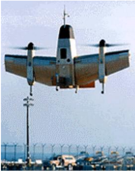
Vertol (Boeing) VZ-2 Tilt Wing VTOL 1959
