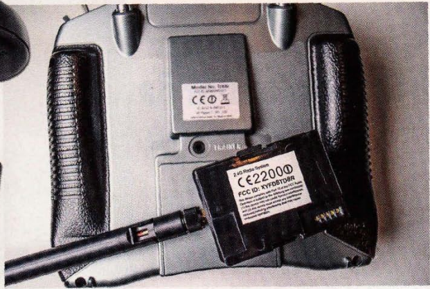
On the backs of my gear are stickers that display the FCC ID code and other product information.
