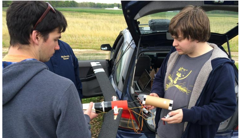
The CG had to be set and checked and the autopilot tumbled through all axes many times to set the range of motions. Then it had to be set level for a few seconds to establish "UP".
