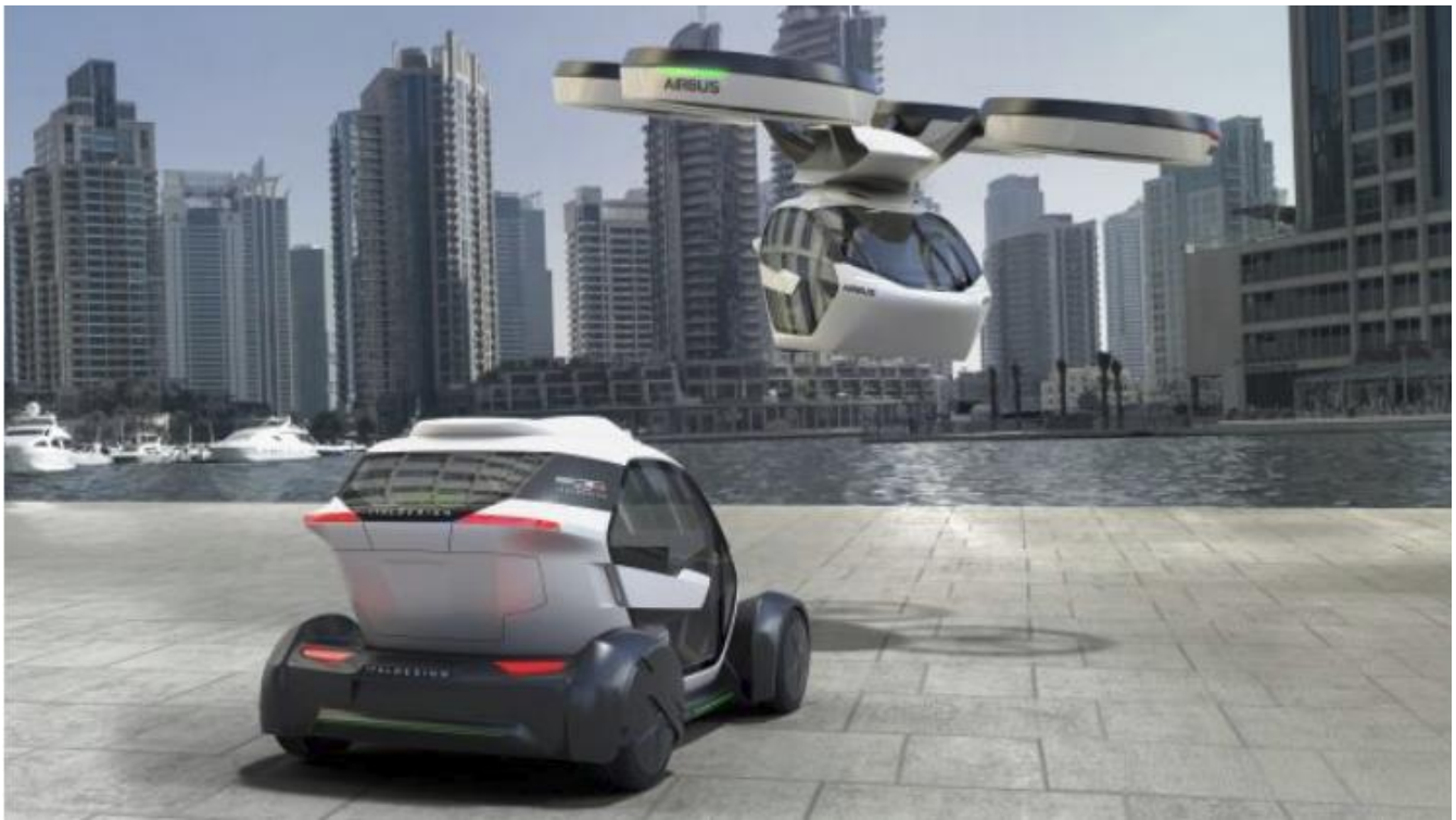
The Airbus/Italdesign Pop.Up comprises a separate aircraft and wheel-base. Credit: Italdesign/Airbus
