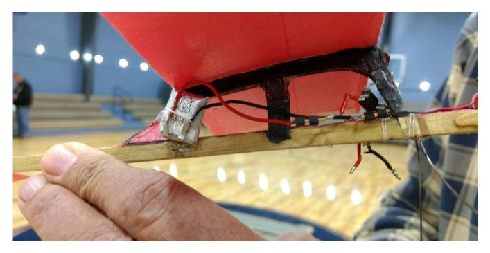
Besides Lipo or Nicad/NiMh batteries there is another choice for us electric motorheads i.e. the high capacity capacitor. My black/white flier uses two capacitors to supply power.
