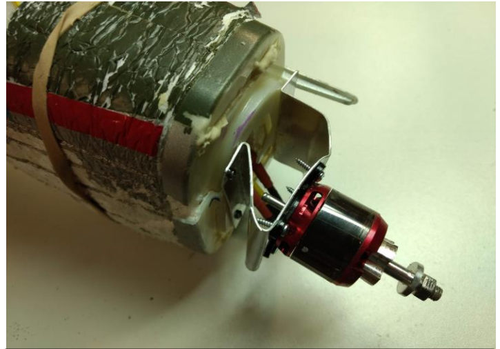
Figure 4. U shaped bracket after crash
