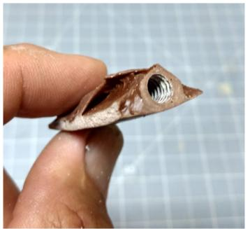
Next I tried it in foam. I drilled a hole in the foam slightly larger than the screw diameter and filled it generously with Bondo, I tied another one later with regular 5 minute epoxy that was equally successful, and then inserted the nylon screw that had been coated with white lithium grease twisting it a little to assure the composite was completely surrounding the screw and filling the void.
