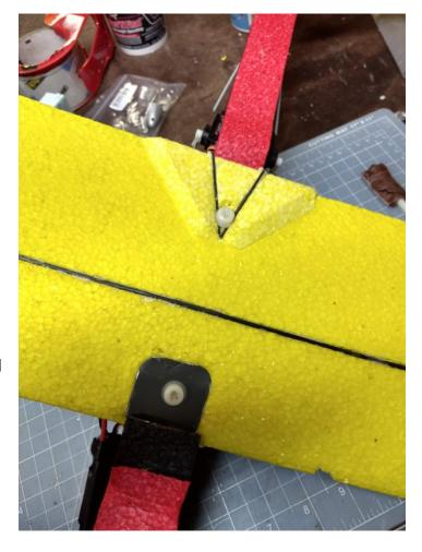
I was faced with this problem recently when planning for the wing saddle connection of a small EPP foam trainer. The entire model was made from wire cut EPP foam. Other than a few pieces of carbon fiber rod reinforcement in the wing and stabilizers and a plywood motor mount, there are no other materials used in the general construction. I wanted a strong, light and simple wing connector.
