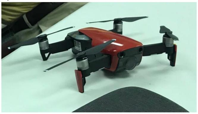
The DJI MAVIC AIR capabilities include a 12 MP camera capable of either still shots or video. This Drone uses a cell phone, which you attach to the transmitter and connect to the aircraft via WIFI, for FPV and to see what the camera is seeing.
