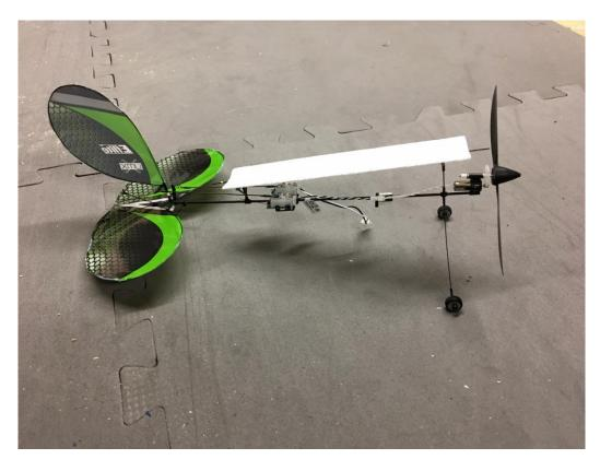
Now the basic airframe weighs about ten grams and the 70mah battery an additional 2.5. So the student's challenge is to design and build a wing in the 5-10 gram range. Dick Bartkowski suggested they use foam from throw away foam plates as being one way to build such a wing. Now just coming up with a wing of suitable size and weight is not enough as it must also have an airfoil which maximizes the lift without adding too much drag.
