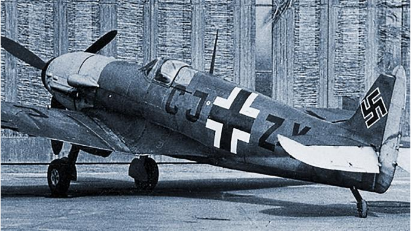
The aircraft mated a Daimler-Benz engine to the body of a Spitfire - THE PRINT COLLECTOR/GETTY IMAGES
