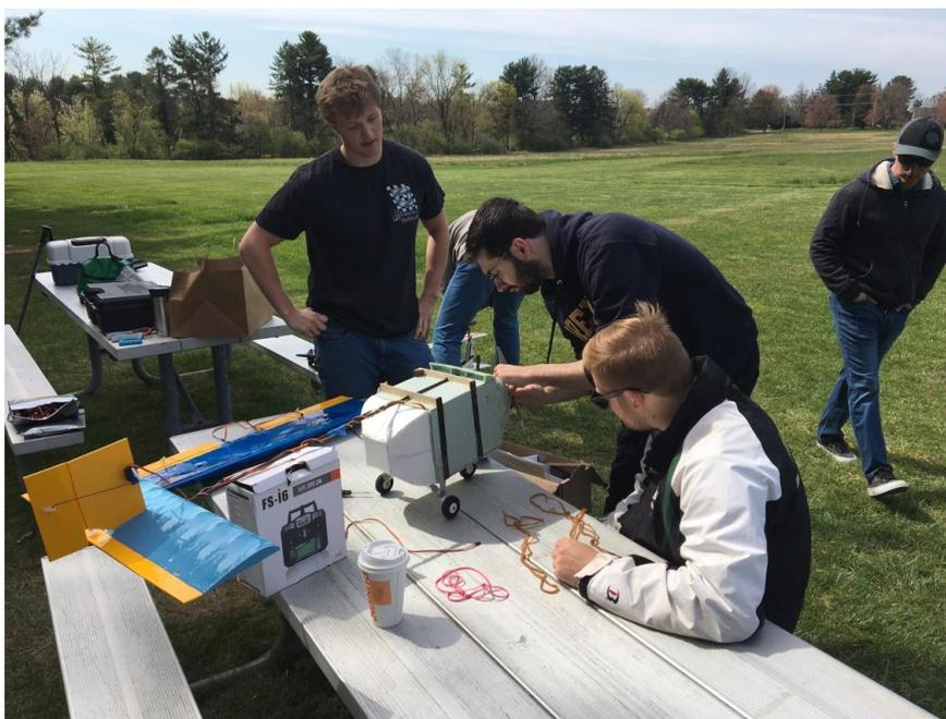
The repair and new motor were not up to the power level of the original and this resulted in a failed table takeoff failure. The local pilot claimed inadequate pitch control to stop the dive off the end. But examining the video it seems more like there was insufficient power as the model just dived off the end indicating no effective aerodynamic lift.
