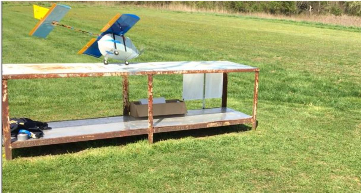
It apparently failed as the torque from this propulsion system overwhelmed the landing gear resulting in a powered roll off the table. So once again the model was taken back to the workshop and repairs made. Oh, this was the day before the teams flew to Texas.
