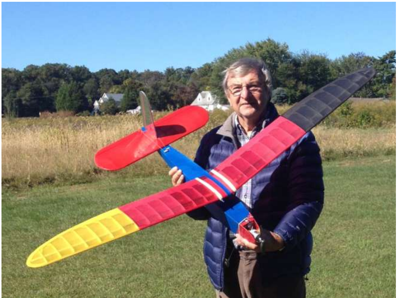
Editor Dave with his new 1/3 scale Boehle Giant test flown and ready to be packed for the flight to California and then on to Las Vegas and the El Dorado Dry Lake for the 2015 SAM Champs. The model will be flown in two events, A Texaco with his 1962 AM 10 diesel engine and Speed 400 with a venerable Mabuchi 400 brushed electric motor. The full sized Giant is already on the West Coast along with the Weather's Westerner powered by a 1935 Brown Jr. Ignition engine and the TU-ANT-25 Scale model.
