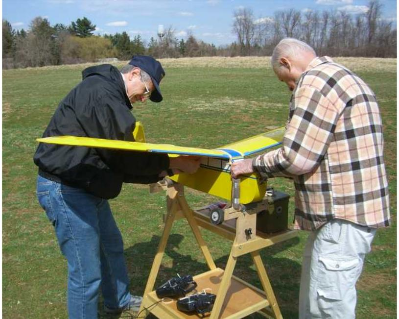
Mike Black and Jim Barrows continue Jim's training on his electric powered Trenton Terror, last year's club model. Jim is using the A123 battery cells and has made five four-cell packs from DeWalt tool batteries. AXI outrunner powered the model has adequate performance but was originally a bit of a handful. So a consultation took place and wise old owl input solicited. A little shim under the back of the wing helped a lot.
