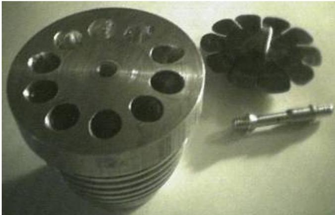
This is a picture of a valve assembly from a Dynajet together with the fuel feed tube. The picture on the right is of the air/fuel assembly from Mick's engine. It is complete and ok.
