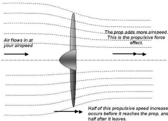
If the air has to be accelerated in order to make thrust, then the speed of the air in the slipstream behind the prop MUST be faster than the airspeed of the rest of the airplane. This speed difference is what we loosely refer to as "slippage".
