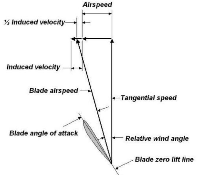
As the plane accelerates, the plane's airspeed increases, so that leg of the triangle increases. This increases the angle between the hypotenuse and the tangential velocity leg, which therefore reduces the difference between that angle and the pitch angle of the airfoil. The angle of attack that local airfoil sees is reduced.
