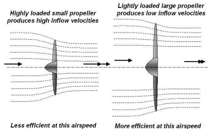
We can also infer from this that when we are trying to absorb a lot of power, make a lot of thrust and/or operate at low airspeeds (such as takeoff and climb), the efficiency of a given prop will not be as good as it is for lower powers and higher speeds (such as cruise).
