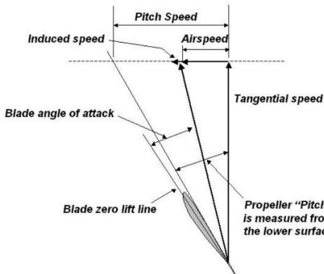
Now let's put some numbers into all this. In the table over leaf are the blade pitch angles for various propellers. We use the definition pitch-to-diameter ratio: P/D, for the propeller because it is this ratio that determines the blade angles.
