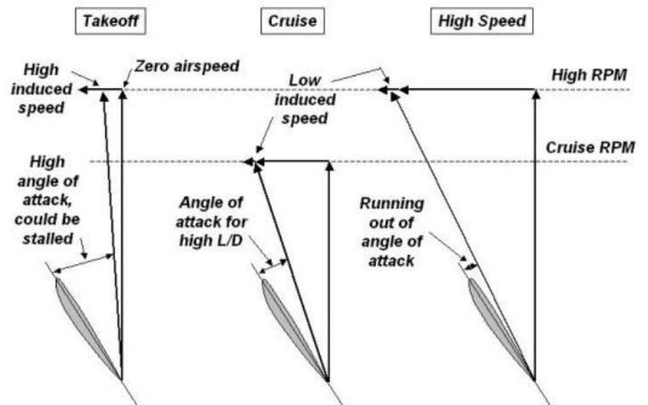
At higher airspeeds, there is more air flowing through the prop, so that air needs less acceleration to convert the power into thrust. This means lower lift coefficients, and therefore lower angles of attack. At the highest speeds the increased airspeed causes the prop angle of attack, and thrust to reduce until thrust equals drag at maximum speed.
