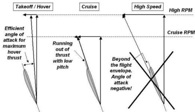
If we select our propeller to match the high-speed flight performance we may not be able to take off due to the propeller operation in deep stall, although the cruise condition may be efficient.
