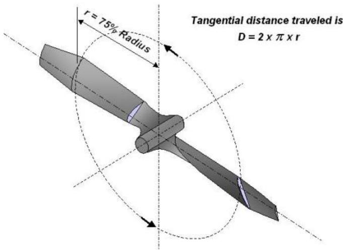
If we multiply that by the revolutions per second that the prop is spinning, we get the velocity in the plane of the prop disk of that location on the blade. We call this the "tangential velocity".
